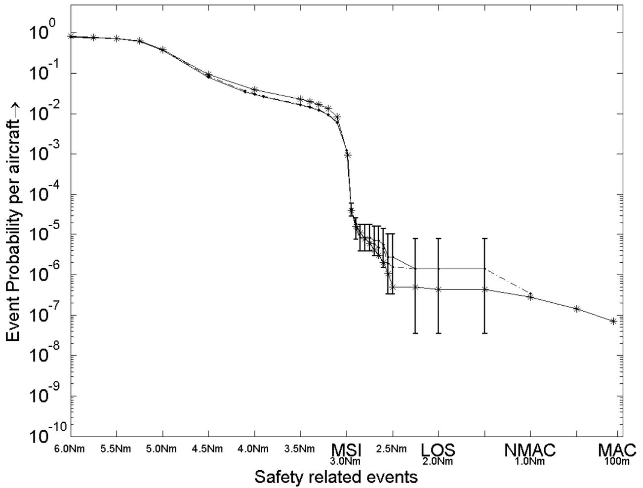
**FIGURE 19:** Standard MC for varying Groundspeed values. \* = standard MC results scenario 0 (baseline), . = standard MC results scenario 6 with 95% uncertainty interval with solid line is estimate using data of Ac1, dashed line is estimate using data of all aircraft.
