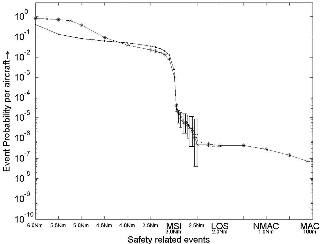
**FIGURE 17:** Standard MC for varying 4D trajectory separation values. \* = standard MC results scenario 0 (baseline), . = standard MC results scenario 4 with 95% uncertainty interval. Solid line is estimate using data of Ac1, dashed line is estimate using data of all aircraft.
