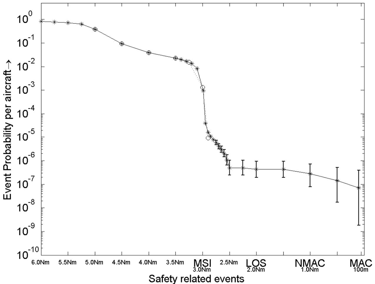
**FIGURE 13:** Standard MC versus IPS based SMC for eight aircraft encounter under A3 and baseline parameter values. Estimated probabilities of safety related events per aircraft in the eight-aircraft encounter. \* = standard MC result estimate using data of Ac1, ○ = sequential MC results. The vertical line segments show the 95% uncertainty interval of the standard MC results.
