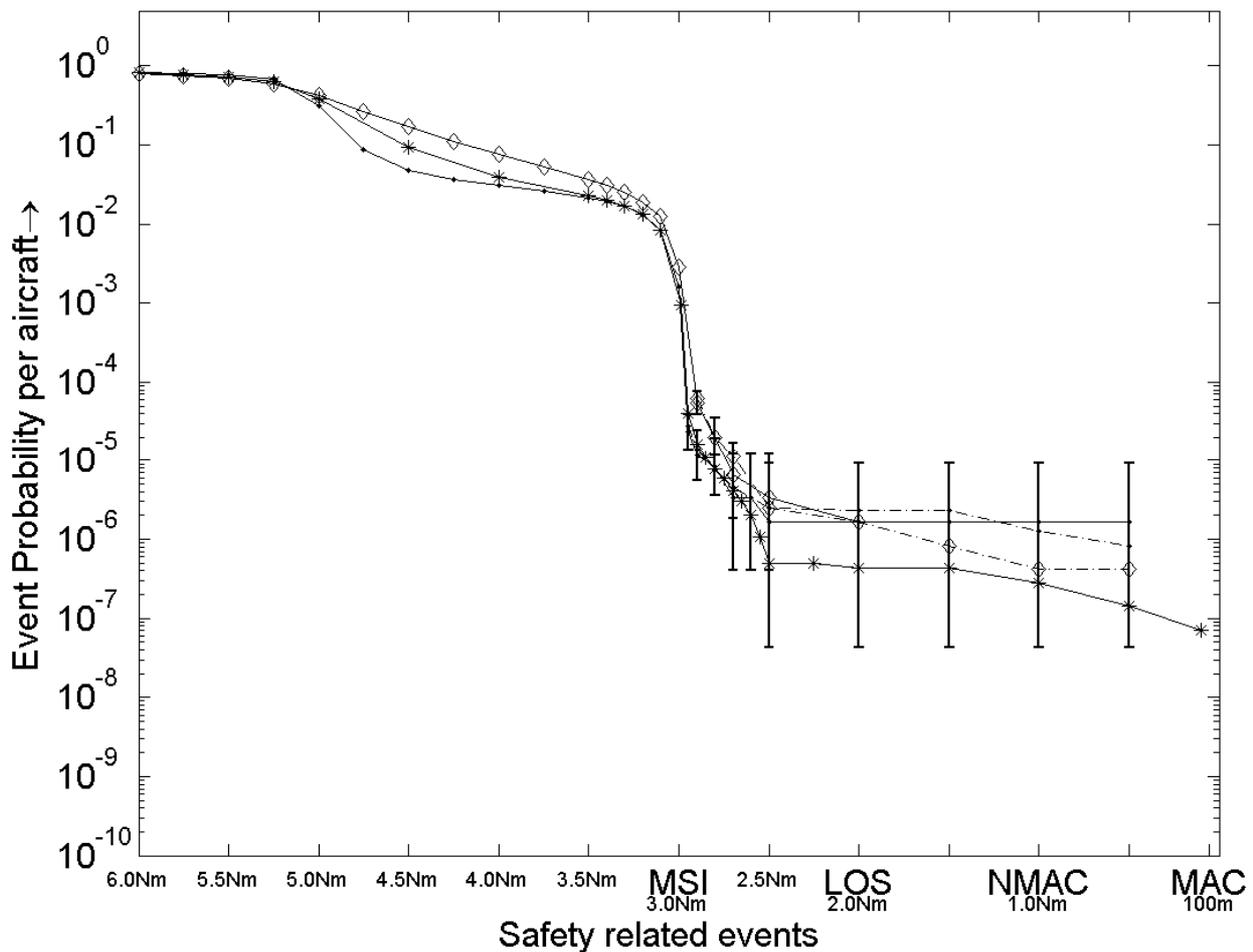
**FIGURE 16:** Standard MC for varying ANP values. \* = standard MC results for ANP1 (baseline),  $\diamond$  = standard MC results scenario 3 for ANP2, . = standard MC results scenario 3 for ANP0.5. Solid line is estimate using data of Ac1, dashed line is estimate using data of all aircraft. The vertical line segments show the 95% uncertainty interval for the Ac 1 estimates.
