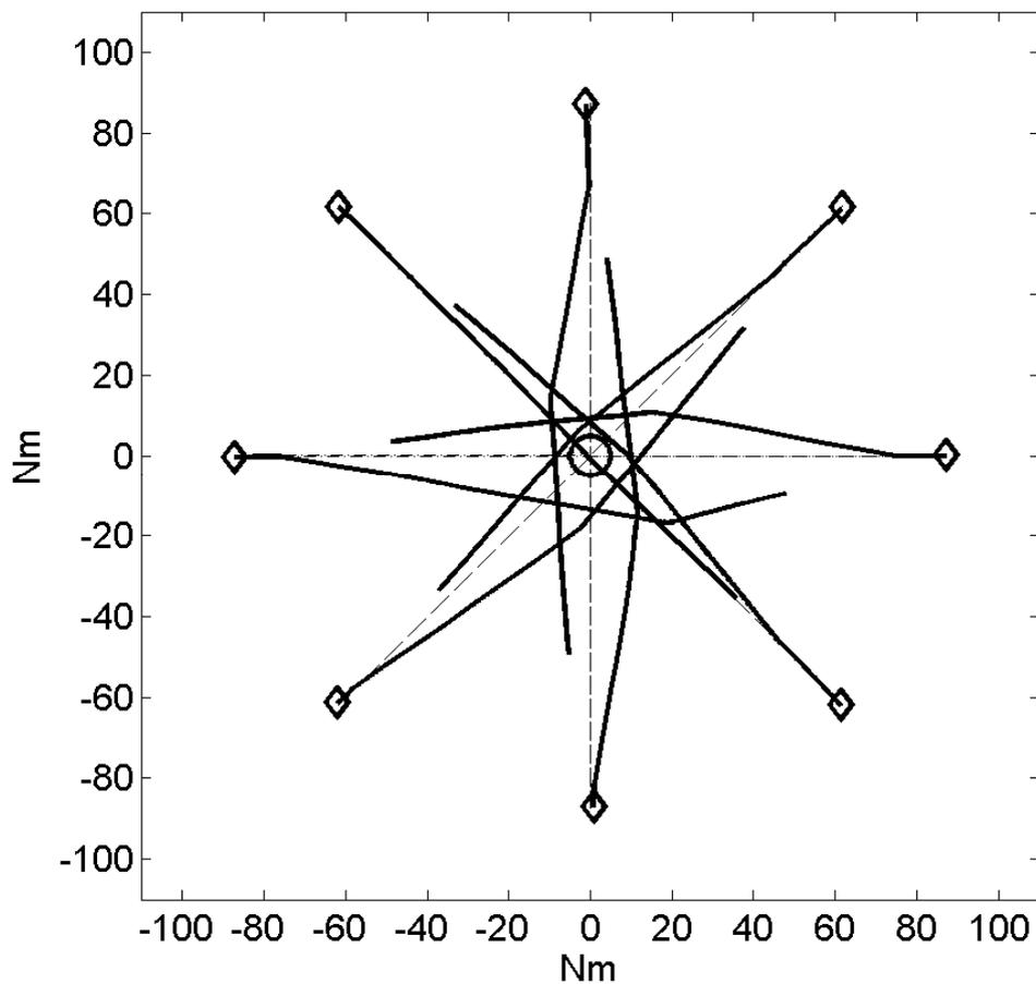
FIGURE 12: A<sup>3</sup> generated conflict resolutions example for eight aircraft encounter scenario;  $\diamond$  = start of simulated trajectory. The circle in the centre has a 10Nm diameter.
