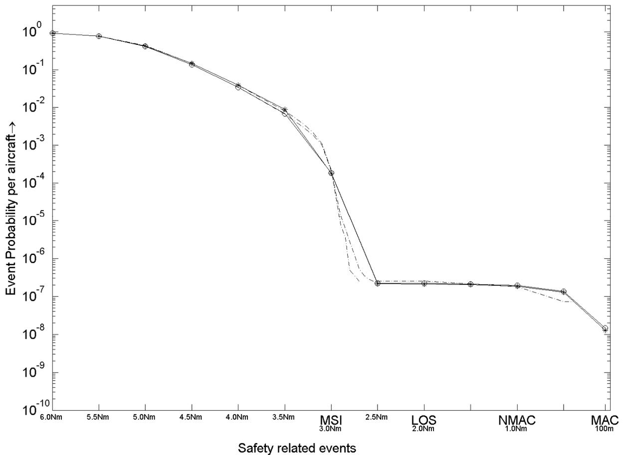
FIGURE 5: Standard MC versus HHIPS based SMC for Varying Crew Response values. Estimated event probabilities for scenario 1.0 and 1.1. ○ = sequential MC results scenario 1.0 (baseline), \* = sequential MC results scenario 1.1, - . = standard MC results.
