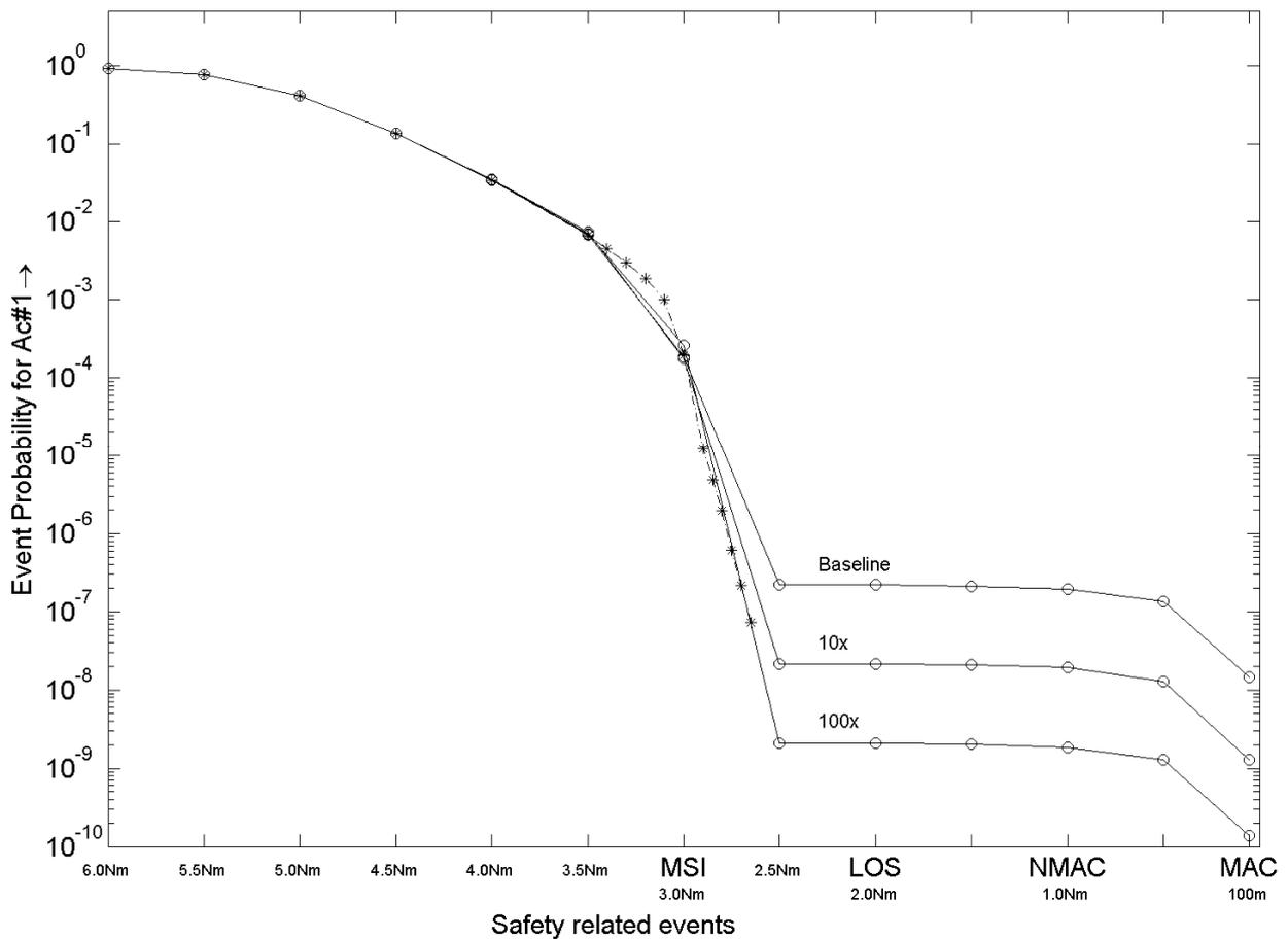
**FIGURE 6:** Standard MC versus HHIPS based SMC for varying Dependability levels. The standard MC simulation results are for the 100x better dependability values only. Estimated event probabilities for scenario 1.0 and 1.2. ○ = sequential MC results, \* = standard MC results.
