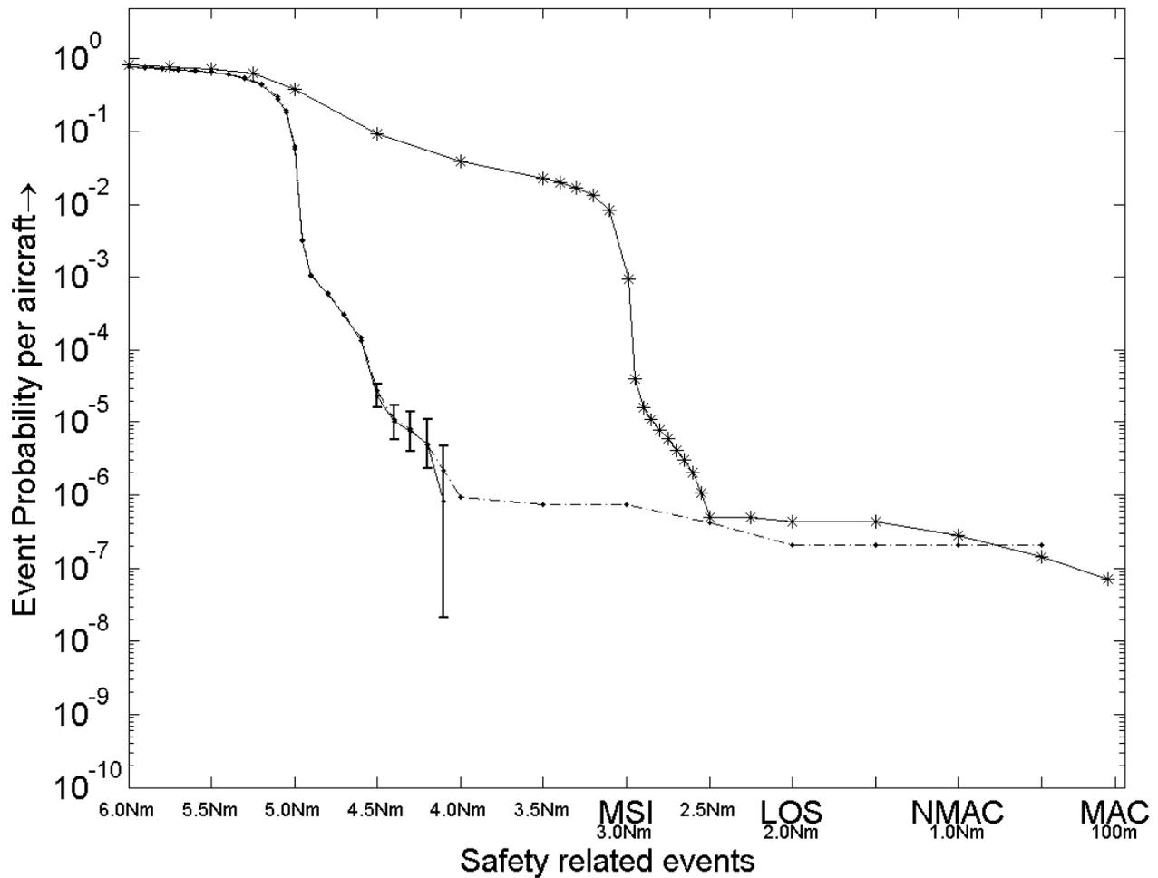
**FIGURE 18:** Standard MC for varying tactical separation values. \* = standard MC results scenario 0 (baseline), . = standard MC results scenario 5 with 95% uncertainty interval with solid line is estimate using data of Ac1, dashed line is estimate using data of all aircraft.
