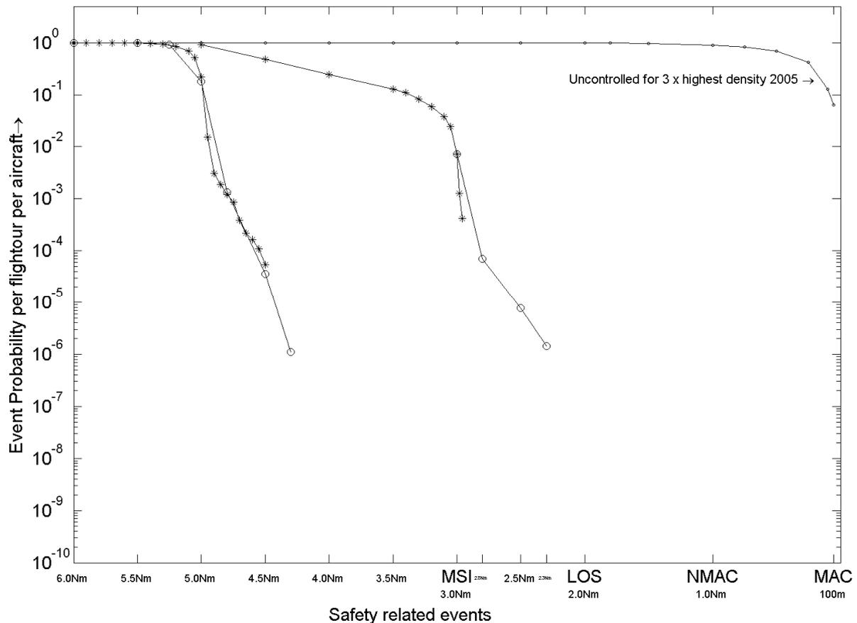
FIGURE 21: Estimated event probability per aircraft per flightour for random traffic under  $A^3$  model control and uncontrolled. Traffic densities is 3x high en-route traffic density in 2005. \* = standard MC, ○ = sequential MC results. Left curve is for tactical separation criterion of 5Nm, right curve for tactical separation of 3 Nm (baseline).
