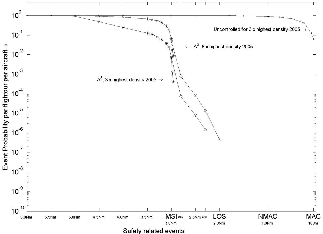
FIGURE 20: Standard MC and IPS based SMC estimated event probability per aircraft per flight hour for random traffic, both uncontrolled and under A<sup>3</sup> model control (baseline parameter values). Traffic densities are 3x and 6x high en-route traffic density in 2005. \* = standard MC result estimate, ○ = SMC results.
