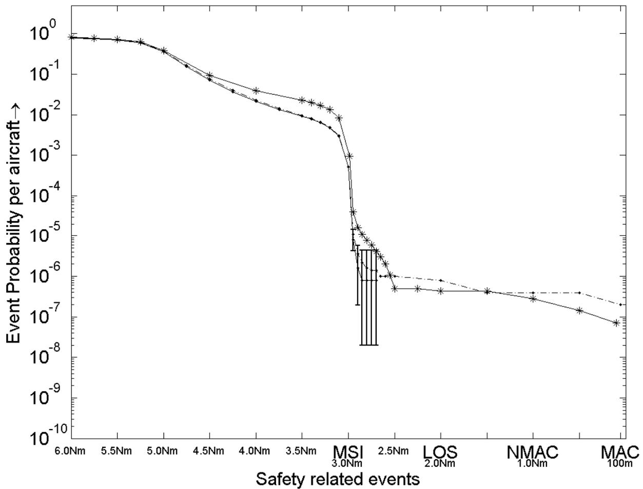
**FIGURE 14:** Standard MC for varying crew response values. \* = standard MC results scenario 0 (baseline), . = standard MC results scenario 1 with 95% uncertainty interval with solid line is estimate using data of Ac1, dashed line is estimate using data of all aircraft.
