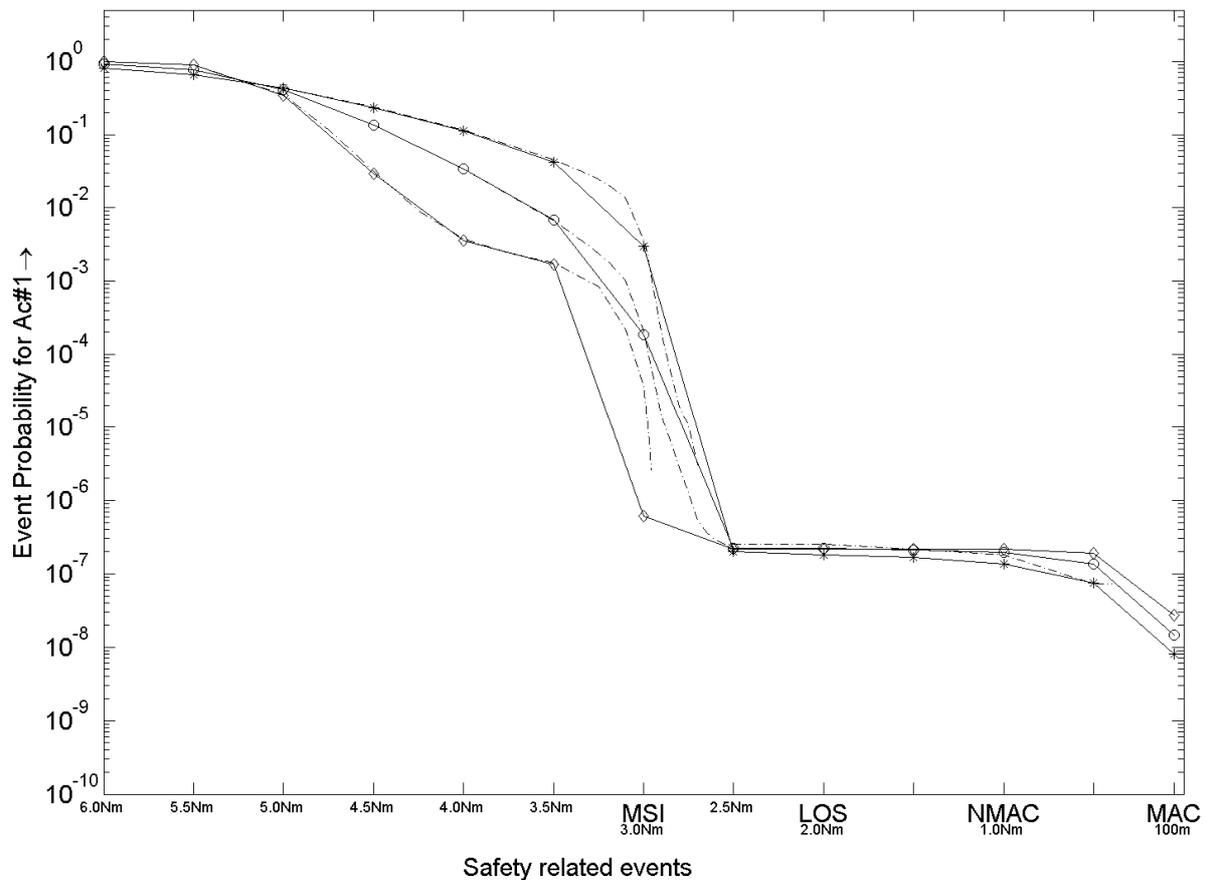
**FIGURE 7:** Standard MC versus HHIPS based SMC for varying ANP values. For ANP0.5 and ANP2, the number of MC runs has been much lower than for ANP1. ○ = sequential MC results scenario 1.0 (baseline), \* = sequential MC results scenario 1.3 for ANP2, ◇ = sequential MC results scenario 1.3 for ANP0.5, -. = standard MC results for ANP0.5, ANP1 and ANP2 respectively.
