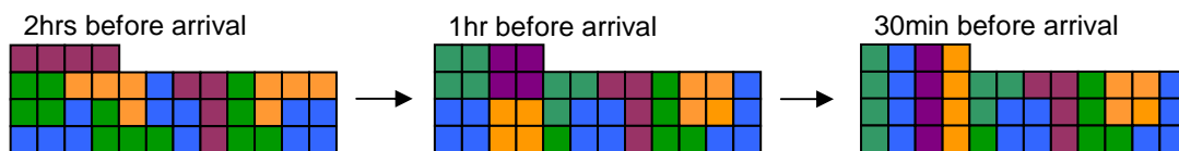
Figure 23 The flexible slot schedule for a specific airspace cell is updated regularly reflecting new information on the time flexibility of the flights.
