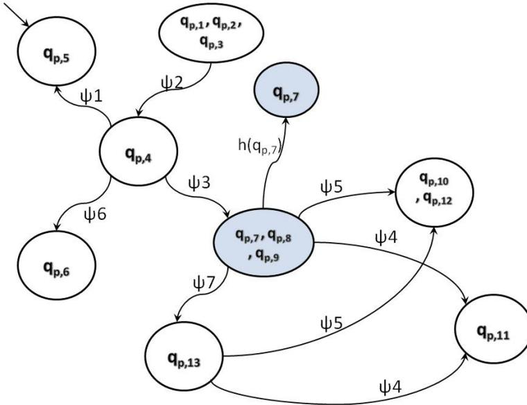
**Figure 5.24:**  $\{q_{p,\tau}\}$ -critical observer with delay for  $\mathcal{H}_p$ .
