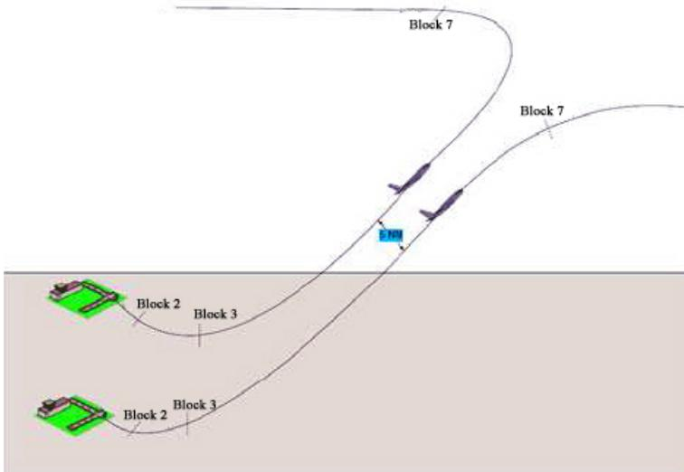
**Figure 5.2:** Encounter type 1. The distance between the route lanes is 5 NM and the radar separation minimum is 3 NM.
