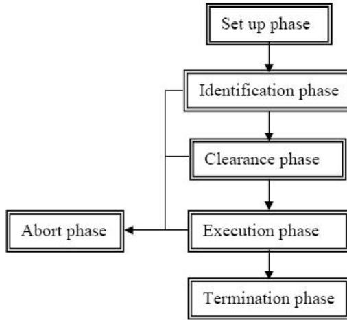
**Figure 5.31:** Phase diagram for ASAS Lateral Crossing procedure.
