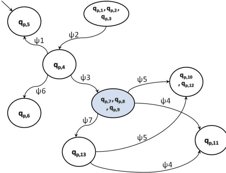
**Figure 5.23:**  $\{q_{p,7}\}$ -critical observer for  $\mathcal{H}_p$
