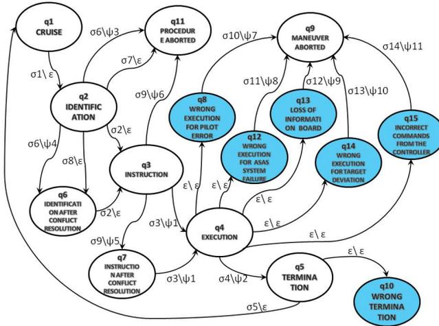
**Figure 5.32:** Hybrid system of the clearance aircraft.
