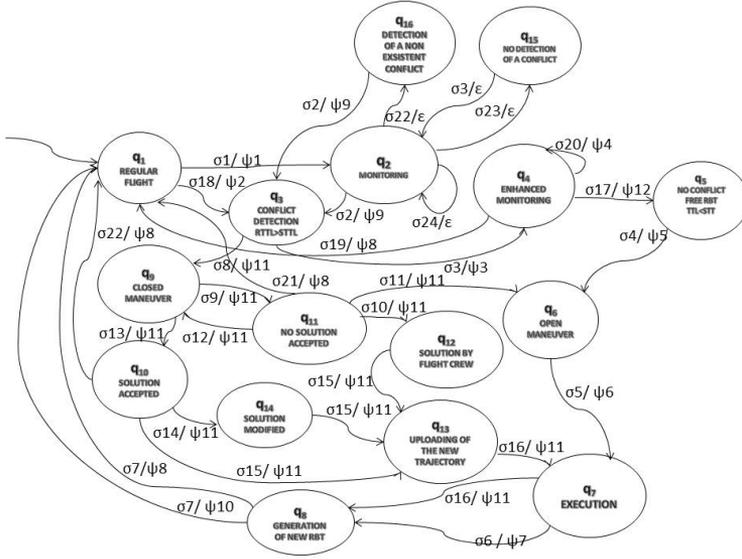
**Figure 5.35:** Hybrid system of the aircraft in nominal conditions.
