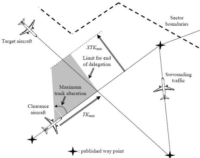
**Figure 5.30:** ASAS Lateral crossing: ATCo perspective.
