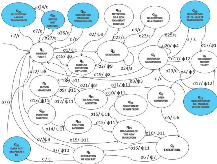
Figure 5.36: Hybrid system of the aircraft in nominal and non-nominal conditions.
