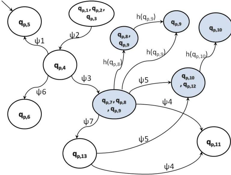
**Figure 5.22:**  $\mathcal{R}_p$ -critical observer with delay for hybrid system  $\mathcal{H}_p$ .
