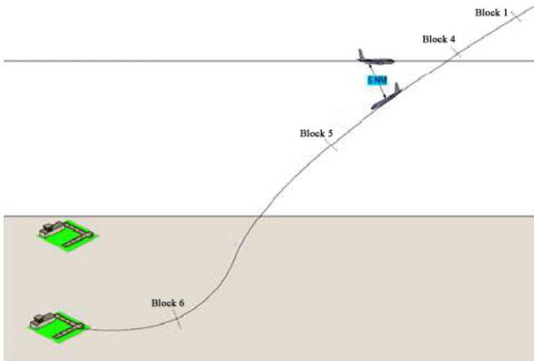
**Figure 5.4:** Encounter type 3. The distance between the route lanes is 5 NM and the radar separation minimum is 3 NM.
