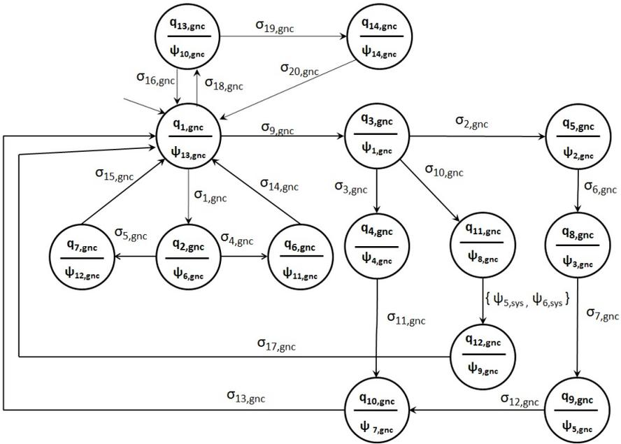
Figure 5.11: FSM for guidance navigation and control agent
