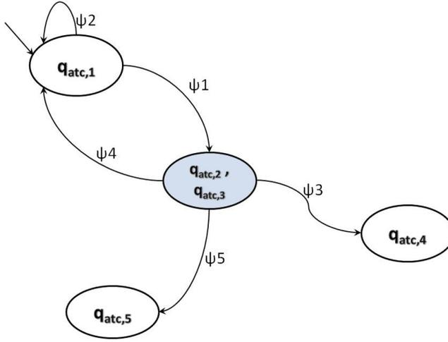
Figure 5.25:  $\{q_{atc,3}\}$ -critical observer for  $\mathcal{H}_{atc}$ .
