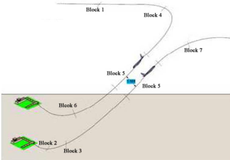
**Figure 5.3:** Encounter type 2. The distance between the route lanes is 5 NM and the radar separation minimum is 3 NM.
