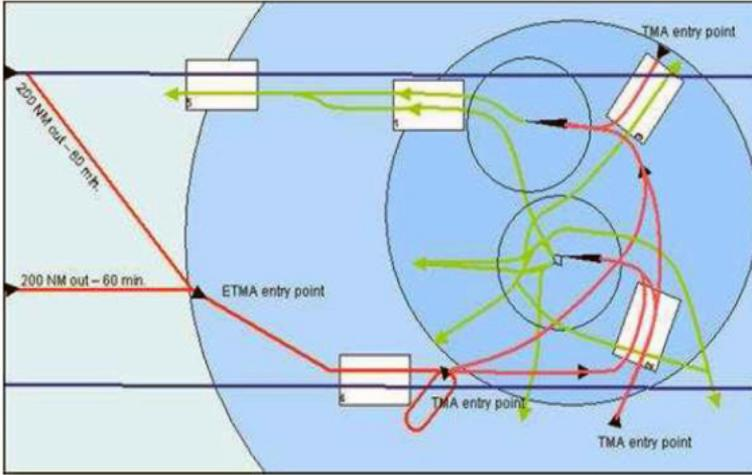
**Figure 5.1:** Example of extended TMA (ETMA) and TMA with entry points and several SIDs (green), STARs (red) and cruise routes (blue).
