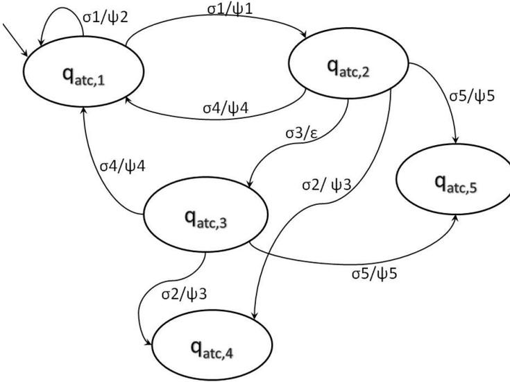
Figure 5.19: Directed graph of the Air Traffic Controller.
