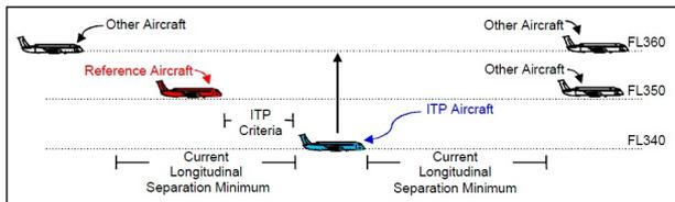
**Figure 5.16:** Example of ITP geometry
