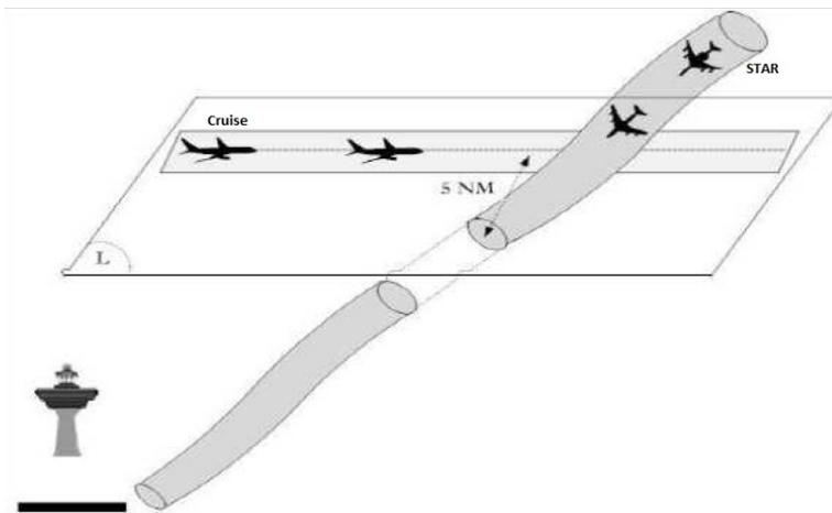
Figure 5.6: Encounter type considered with aircraft on a STAR and aircraft en-route
