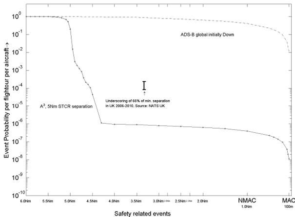
Figure 10. Estimated event probability per aircraft per flight hour for random traffic under  $A^3$  model control at traffic demand of 3x high en-route traffic demand in 2005. The dashed curve at the top is obtained through running standard MC simulations for the  $A^3$  ConOps model under the initial condition that ADS-B Global is Down. nd uncontrolled. This curve has been used to construct a completion of the line curve for miss distance values below 4Nm.
