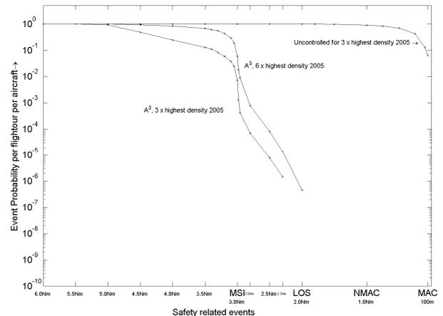
Figure 8. Estimated event probability per aircraft per flight hour for random traffic under  $A^3$  model control and uncontrolled. Traffic densities are 3x and 6x high en-route traffic density in 2005.
