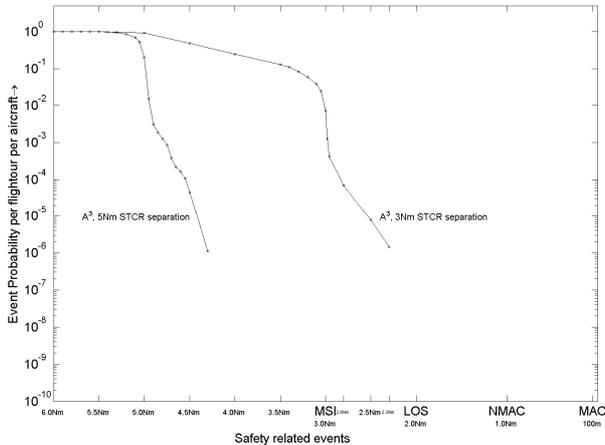
Figure 9. Estimated event probability per aircraft per flight hour for random traffic under  $A^3$  model control at 3x high 2005 en-route traffic demand. Left curve shows effect of 5 Nm STCR separation.
