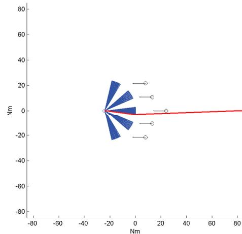
Figure 1. Velocity Obstacles (3 minutes & 3 Nm.) in case of five head on encountering aircraft, together with a conflict free path (red line).
