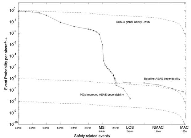
Figure 6. Effect on event probabilities of improving the dependability values for GNSS, ADS-B and ASAS systems by a factor 100x. The dashed curve at the top of the Figure is obtained by running standard MC simulations for the case that ADS-B is initially Down. The other two dashed curves copy the top level curve down at factors  $10^{-6}$  and  $10^{-8}$  respectively.
